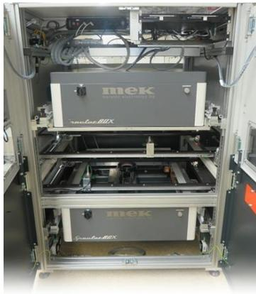
The Mek SpectorBOX broke new ground in AOI when it was introduced several years ago. Its unique look up and look down capabilities made it an instant hit for THT inspection, eliminating the need for board flipping while providing the ability to examine every defect in microscopic detail.
