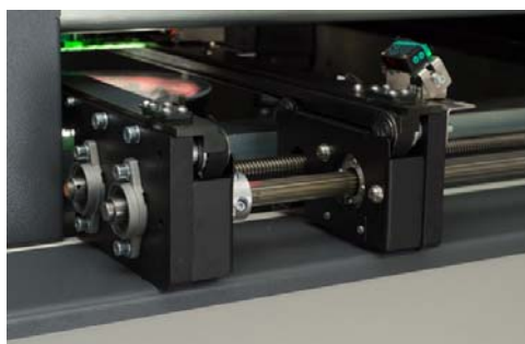
Adjustable width tooth belt conveyer transports assemblies up to 15kg. Equipped with optical stoppers
