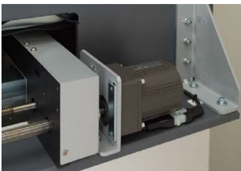
Levelling brackets for easy adjustment of the SpectroBOX focus and conveyer height. The levelling brackets allow single-person easy levelling, even with pre-mounted SpectroBOXes. Built-in mm-rulers integrated in the mainframe poles, allow easy pre-adjustment in advance of final levelling. The Top rail can hold an additional SpectroBOX for Top Down inspection. Equipped with the same level brackets to allow easy levelling and pre-adjustment.
