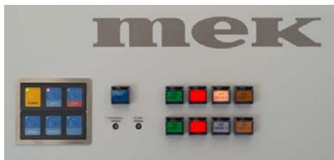
Conveyer operation panel to select operation modes and monitor AOI
