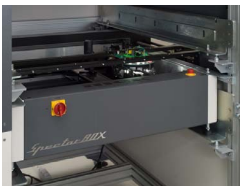
Levelling brackets for easy adjustment of the SpectroBOX focus and conveyer height. The levelling brackets allow single-person easy levelling, even with pre-mounted SpectroBOXes. Built-in mm-rulers integrated in the mainframe poles, allow easy pre-adjustment in advance of final levelling. The Top rail can hold an additional SpectroBOX for Top Down inspection. Equipped with the same level brackets to allow easy levelling and pre-adjustment.
