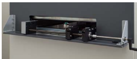
Conveyer entries can be designed upon customer specification with regard to size and safety features. The image shows version with width adjustment via a detachable manual crank
