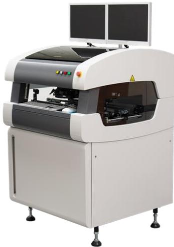
The new [Mek PowerSpector BTL AOI systems](#) offer synchronized inspection of the top and bottom side of PCBs after Reflow, Wave or Selective soldering & placement of SMT & THT components.
