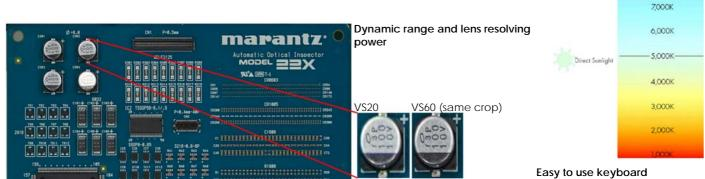
Zoom lens: Adapt your resolution to specification needs With the availability of VS20/40/60 models, three different cameras equipped with a zoom lens, the VeriSpector can be fine-tuned to your inspection requirements or standard Solder Frame dimensions.
