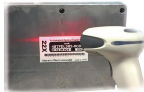
Instantly access to the inspection data or image by reading the barcode on target workpiece with barcode reader.
